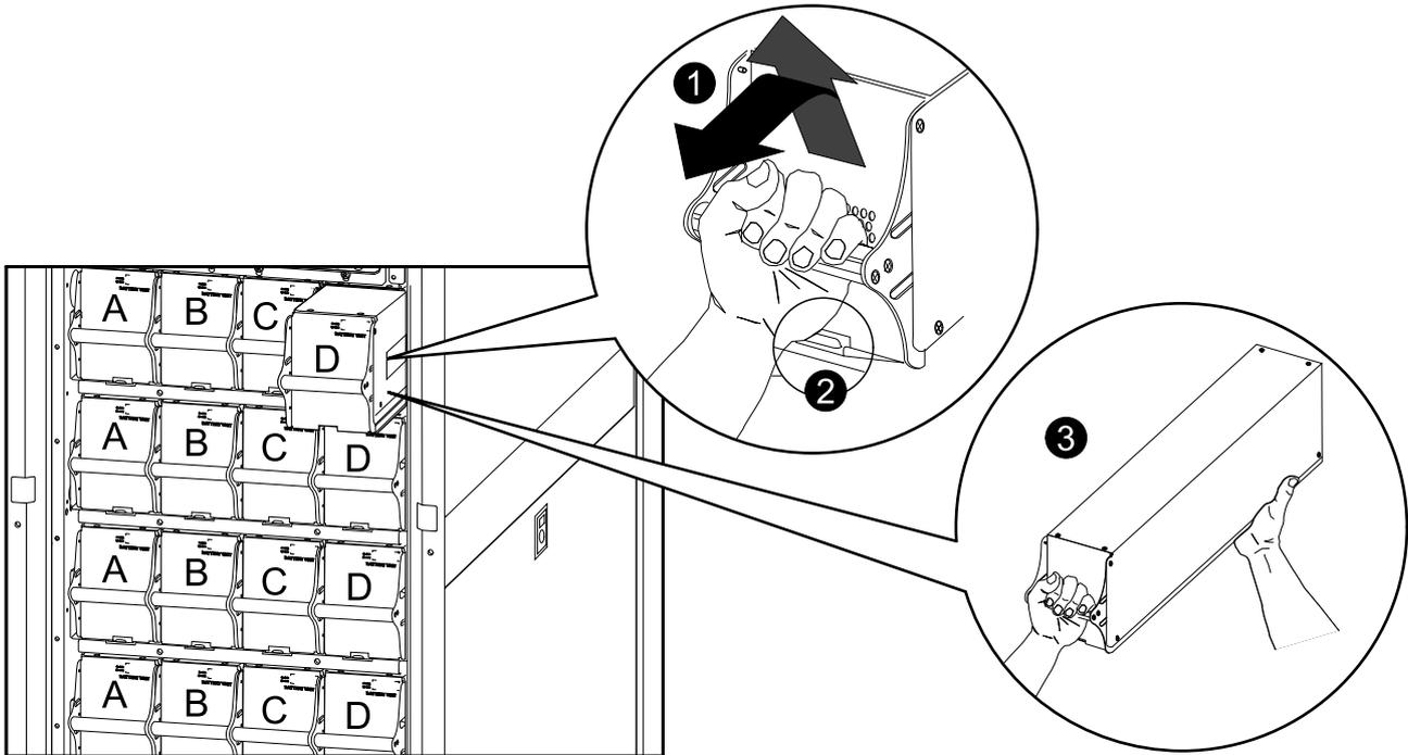
**NOTE:** When removing battery modules, start from the highest level and work down.
