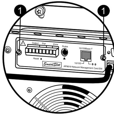
1. Loosen the two Torx screws (one on each side of the card).
