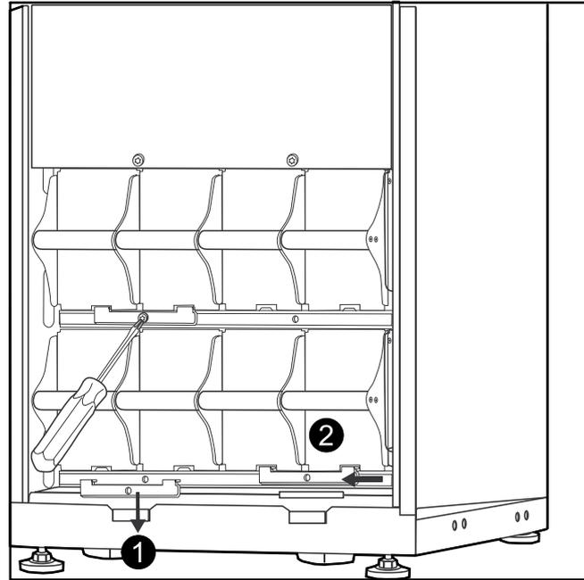
2. Push the battery lock to the left, push it upwards and remove.
