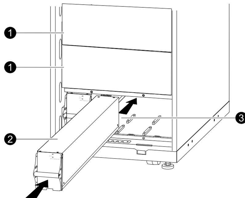
1. Remove the blind plate (if present) in front of empty battery shelves (if present) and save the screws for later use.
