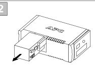
Pull the battery out, exposing the battery terminals and wires. Disconnect the wires from the terminals.
