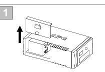
Place the unit on its side. Slide the battery compartment cover upward and off of the UPS.
