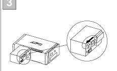
Slide the new battery into the battery compartment.
