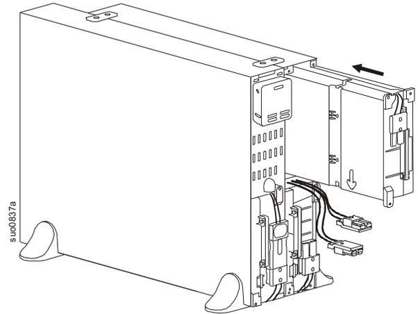
3 Secure the battery modules with the enclosure with 6 screws.
