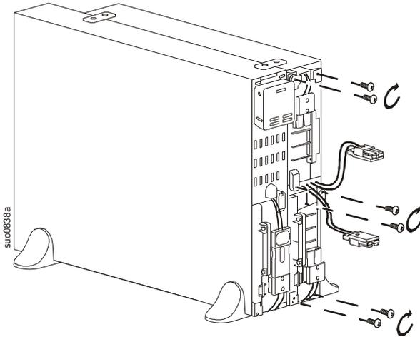
4 Connect the two XLBP connectors from the enclosure to the two RBCs. See “XLBP Connectors Installation” on page 6.
