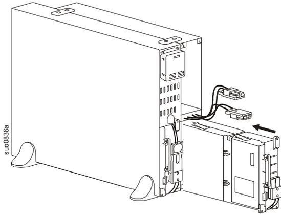
2 Slide the top side battery module into the XLBP.
